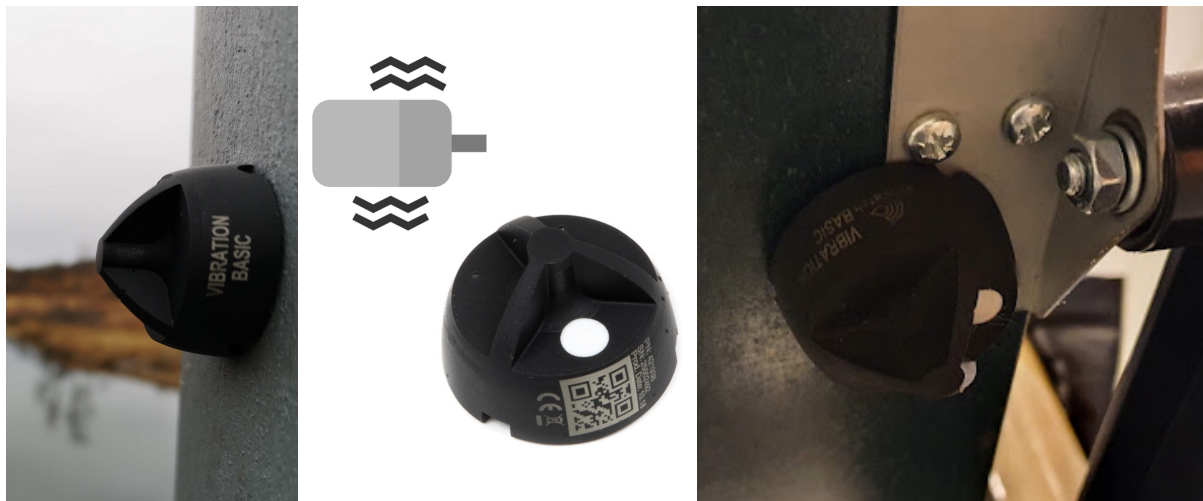
Figure 4.2.6: Vibration sensor mounted on a wall (El-Watch Website 2020) and vibration sensor mounted on tennis table using a magnet (right picture)
